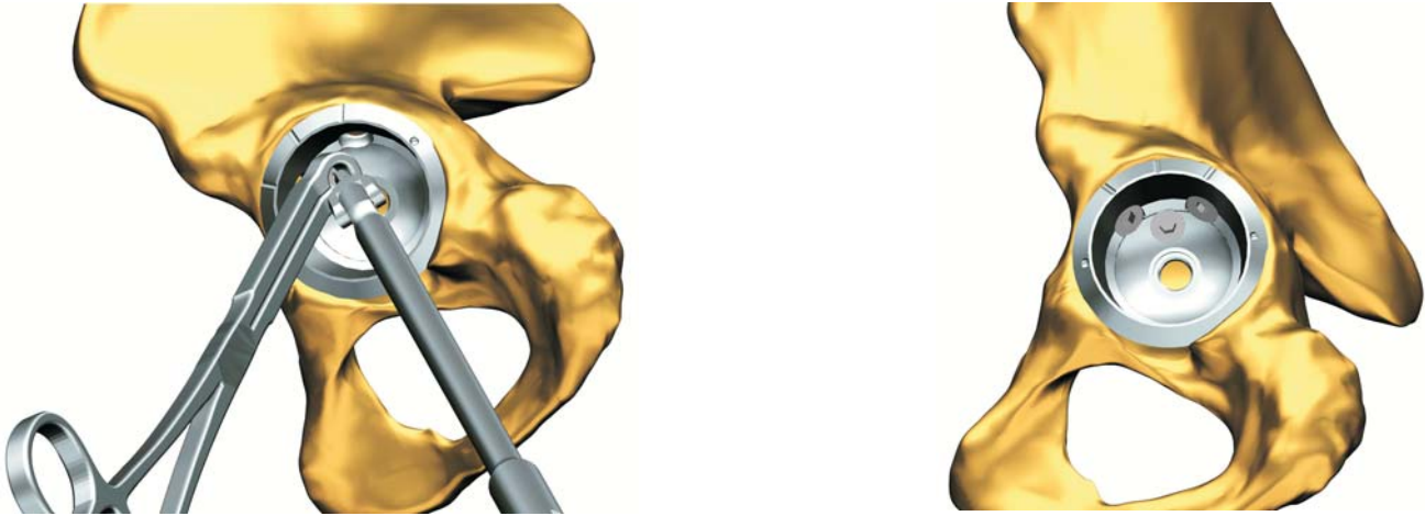
Figure 13: Bone screw insertion (left), verify proper seating after insertion (right).
